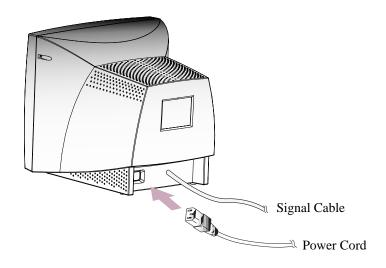
If your power cord is PC-to-Monitor type, plug the other end of the power cord into the AC receptacle in the computer.
